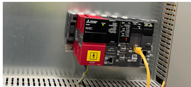
The Melsec I-QR series controller provides the operating data for the Asset Portal via the RD55 data logger. Source: Mitsubishi Electric Europe B.V.
